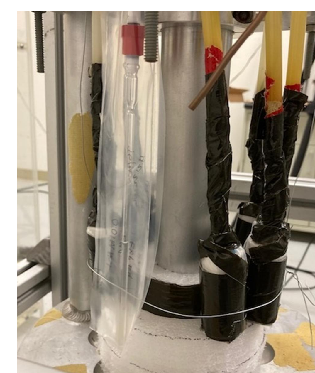
Figure 8. PNNL ^{60}\text{Co} gamma irradiation system.
