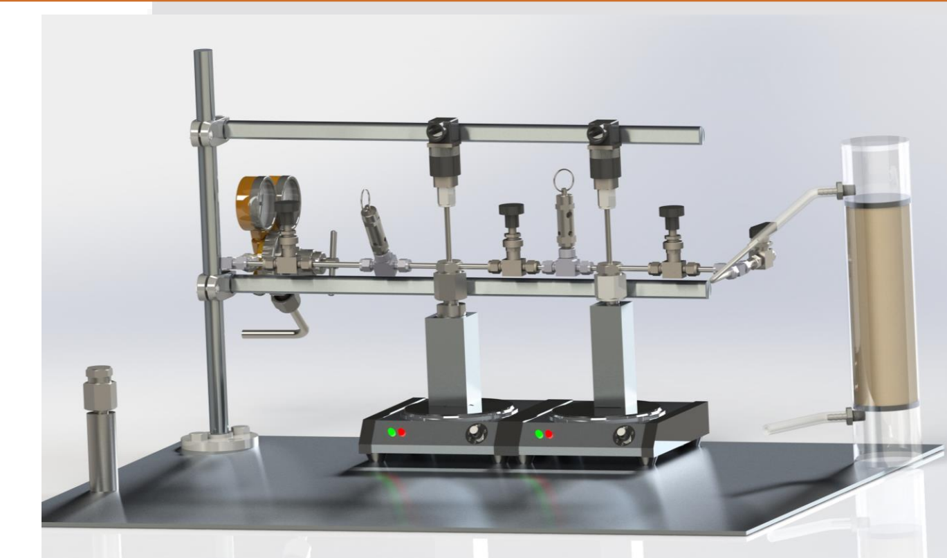
Figure 11. Apparatus to collect thermodynamic data at elevated temperatures
