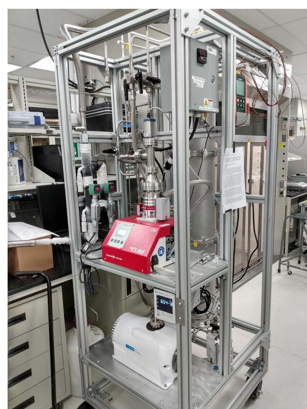
Figure 3. Prototype LN cooled abatement trap
